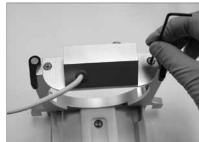
Figure 4A: Removing one of the 6-32 x 5/16" flat head screw securing the electronics housing assembly onto the interface flange
