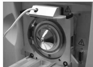
Figure 3B: Interface flange levers are open – the Interface flange is ready to be removed.
