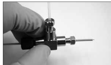
Figure 14B: Sheath gas tee with sheath gas tubing installed.
